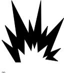
**Batteries can produce explosive gas.** Do not smoke, use open flame, or create an arc or sparks near this battery. Ventilate well when in an enclosed area and when charging.
