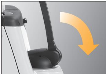
**Note:** Braking is designed to stop your truck in the shortest distance. Use the brake in an emergency, on ramps, or in busy areas.
