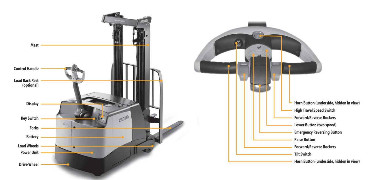
9 Lift Truck Parts Lift Truck Parts 10
