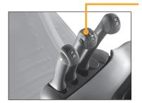
If your truck is equipped with this option, the forks will go to the programmed tilt position chosen by your company for this truck.
