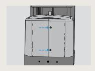
**Note:** Make sure you know your Truck Type. See **Capacity Plate** on page 36. For EE Truck Types, make sure to lock the battery retainer.
