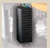
Sealed on-board charger practically eliminates contamination entry which can result in failure. In addition, the charger has been designed to operate without a separate cooling fan for even greater reliability.
