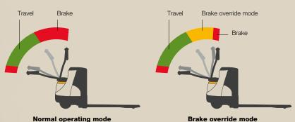
Crown gives operators the best of both worlds: in the **normal operating mode** a large brake zone ensures that operators can easily and quickly stop the truck during normal operation. When working in tight spaces, the **brake override mode** enables operators to position the handle in near vertical position while engaging traction at creep speed for fine-tuned load positioning.
