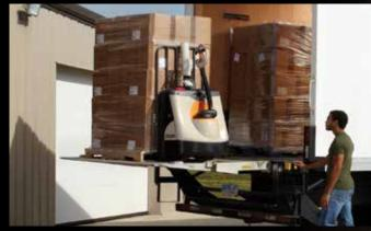
Thousands of applications without receiving/shipping docks require delivery from truck to curb side via lift gates. Crown's compact design, exceptional maneuverability and brake override features make the WP 3000 Series ideal for these applications.
